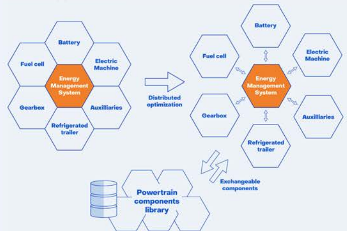
Figure 1: Converting one big optimization problem into smaller optimization problems to allow for complex configurations
