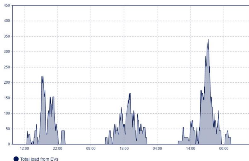
Figure 23, Uncontrolled load profile on transformer based on 165 EVs
