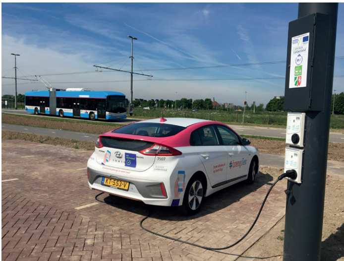
An electric vehicle being charged with power from Arnhem's trolley network (Photo: the municipality of Arnhem)
