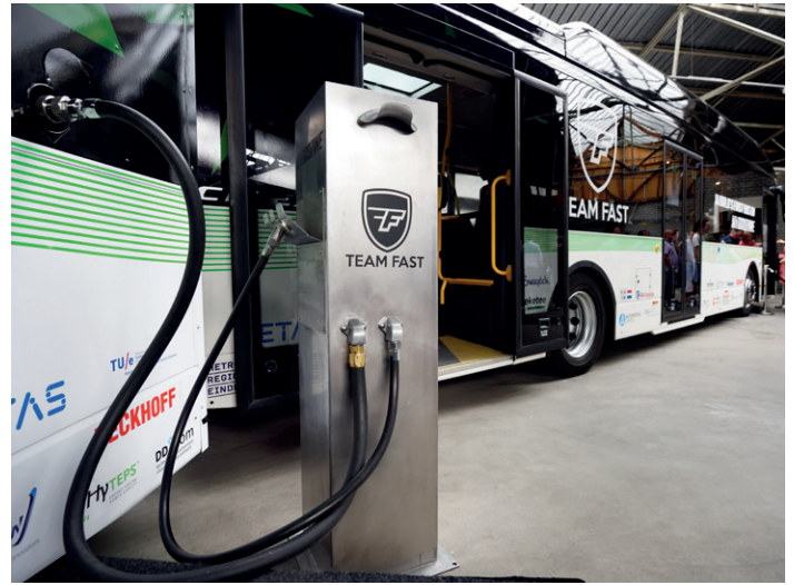
The electric bus that runs on formic acid, developed by Team FAST from Eindhoven University of Technology (Photo: Eindhoven University of Technology)
